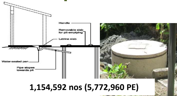
1,154,592 nos (5,772,960 PE) Cess pit (Obsolete)
