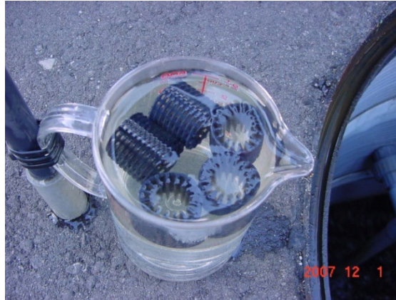
Check condition of biofilm
