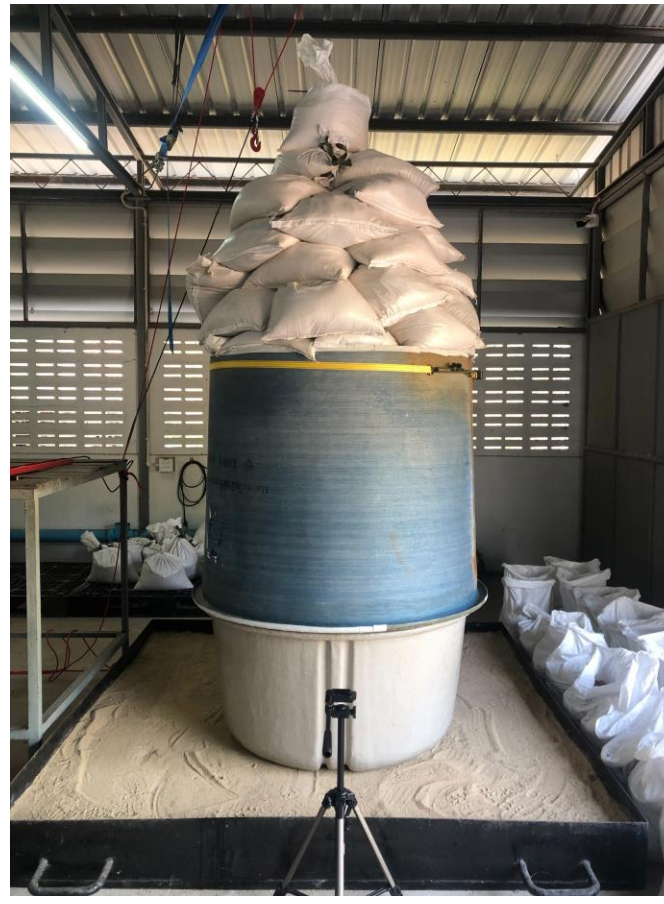
Vertical loading test
