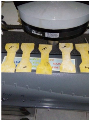
FRP Material test in laboratory of Ministry PUPR
